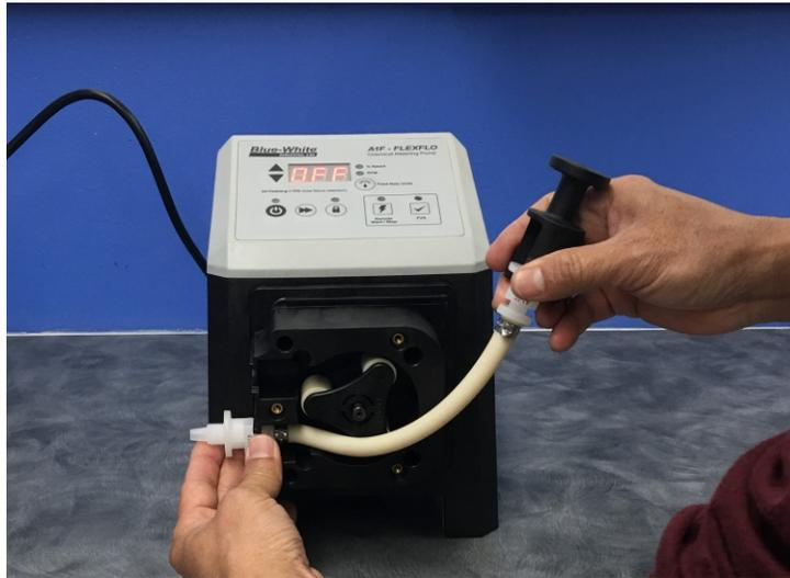
3. Stretch the tube slightly and insert the outlet (discharge) fitting into the upper retaining slot of the pump head. Pull the outlet fitting out of the pump head.
